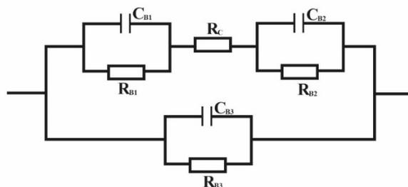
**Figure 5.** Model of the structure of the near-surface region of diffusion -doped silicon with manganese, chromium and cobalt atoms.  $R_C$  – resistance of the compensated area,  $C_B$ ,  $R_B$  – capacitance and resistance of the Schottky barrier, respectively.
