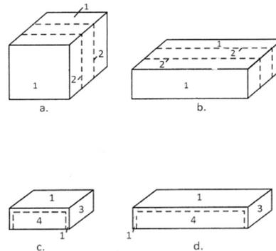
**Figure 1.** Type of sample Si <Mn>, Si<Co>, Si<Cr> for studying photovoltage and photoconductivity:
