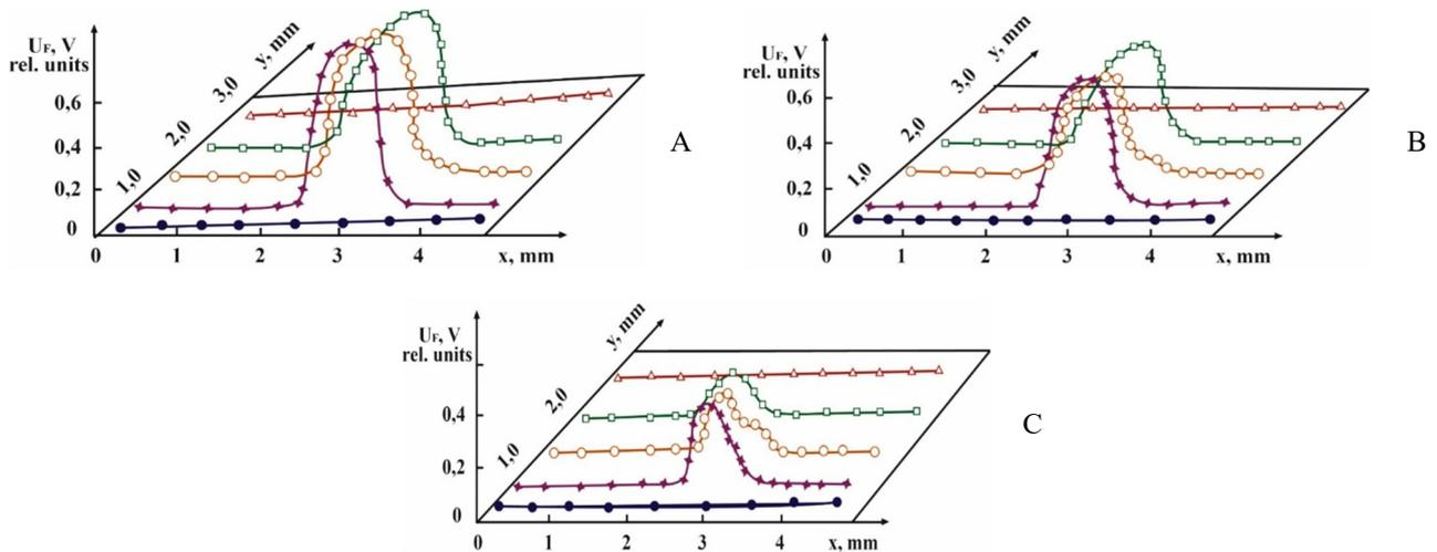
**Figure 3.** Light scanning results for one sample p - Si < Mn > when irradiated with light of different wavelengths:
