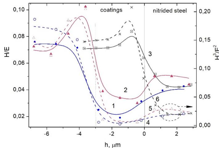
**Figure 4.** Distributions of  $H/E$  and  $H^3/E^2$  ratios across the interlayer boundaries of modified layers using Mo (1, 4) and Ti (2, 5) coatings as well as without metal layer (3, 6). The thicknesses of the layers are: 3  $\mu m$ .
