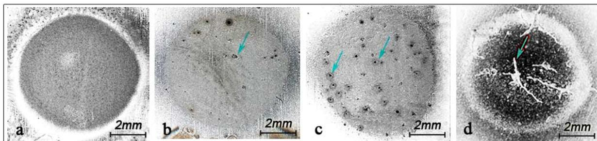
**Figure 6.** Surface microstructure of specimens after 6 h of cavitation tests: untreated steel (a), Mo<sub>2</sub>N coating without interlayer (b), Mo<sub>2</sub>N with 3 μm Mo layer (c) and Mo<sub>2</sub>N with 3 μm Ti layer (d).
