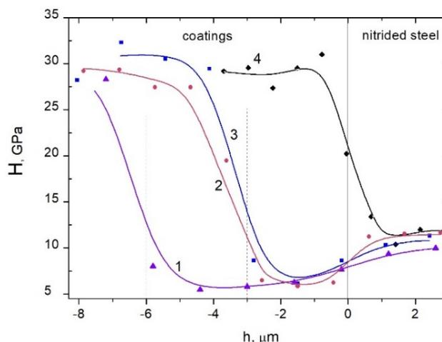
**Figure 2.** Hardness distributions along cross sections of modified coatings with Mo (1, 3), Ti (2) interlayers and no metal layer (4). The layer thicknesses are: 3  $\mu\text{m}$  (2, 3) and 6  $\mu\text{m}$  (1).
