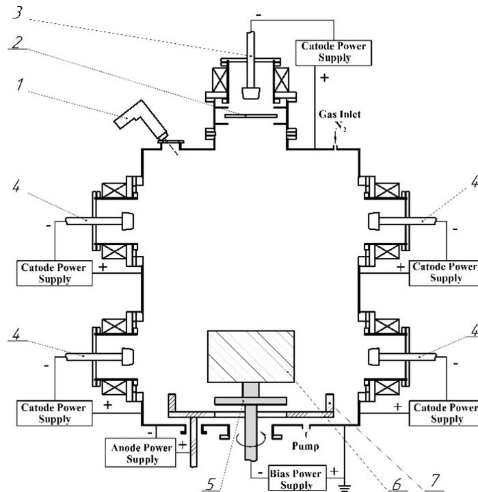
**Figure 1.** Scheme of the experiment: 1 - pyrometer, 2 - shield, 3 - plasma source of the first stage of two-stage discharge, 4 - plasma sources with Mo or Ti cathodes, 5 - rotation device, 6 - model of the part, 7 - electrode of the second stage of discharge
