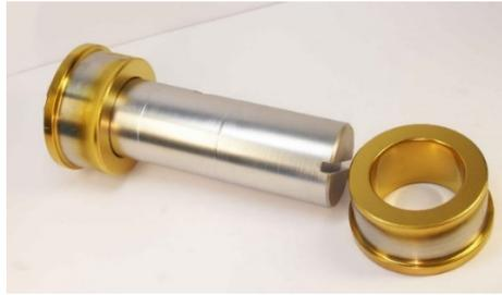
**Figure 8.** Images of parts ("Axis" - in the center and "Insert" - on the edges) of the friction pair included in the steam distribution unit of the K-325 turbine.
