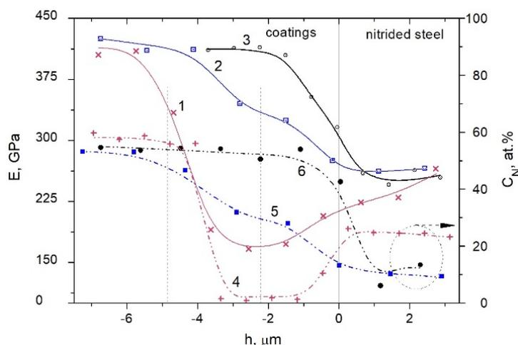
**Figure 3.** Distributions of Young's modulus (1, 2, 3) and nitrogen concentrations (4, 5, 6) along the cross sections of modified layers with Ti (1, 4), Mo (2, 5) and without metal layer (3, 6) coatings. The thicknesses of the layers (1, 2, 4 and 5) are 3  $\mu\text{m}$ .
