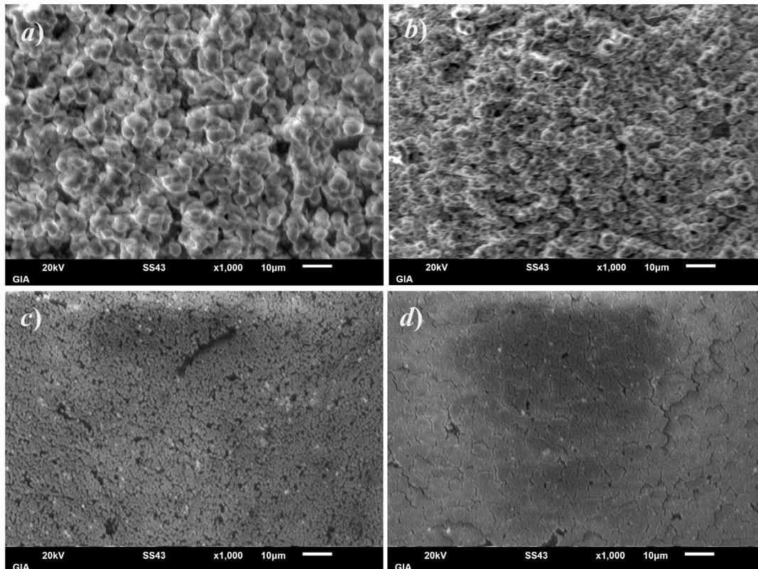
**Figure 1.** Surface structure of thin CdSe films of various thicknesses: *a*)  $h = 200$  nm, *b*)  $h = 300$  nm, *c*)  $h = 400$  nm and *d*)  $h = 500$  nm.
