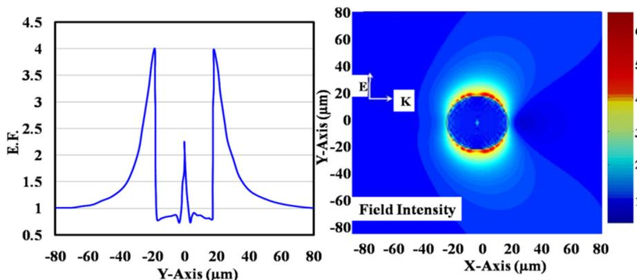
**Figure 3.** Electric field pattern of a 20 nm radius sphere ( $K||X$ ,  $E||Y$ ) on the right, and on the left field enhancement around a nano-sphere along the Y-axis
