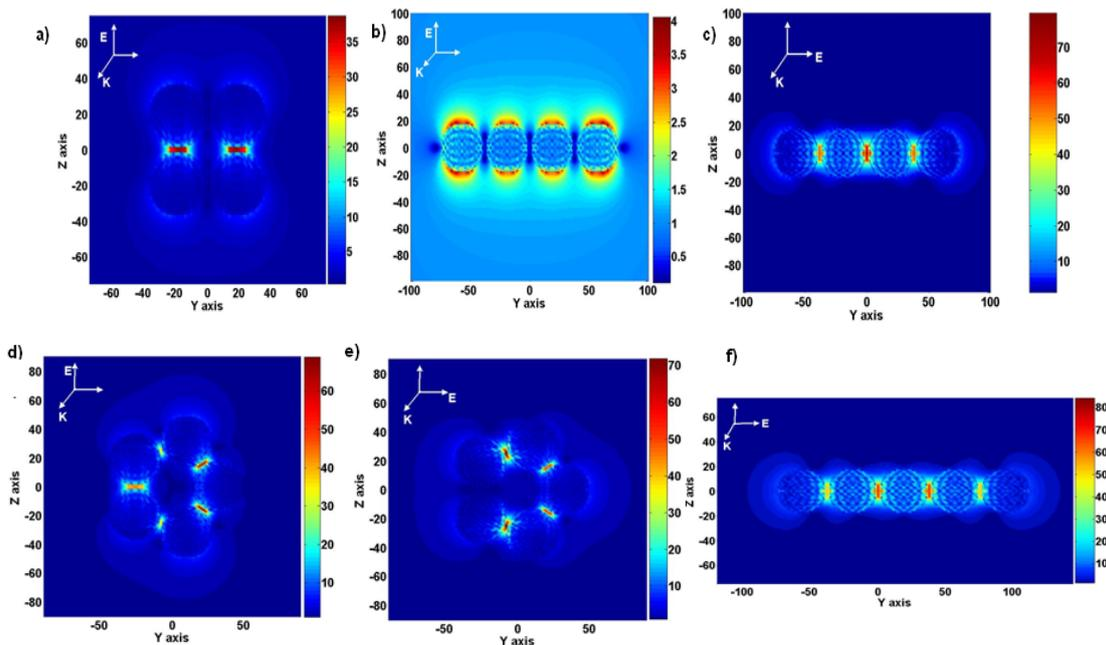
**Figure 7.** Electric field patterns for 4 & 5 spheres in different configurations
