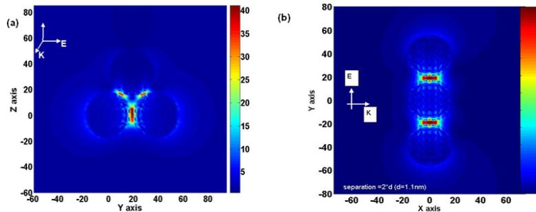
**Figure 6.** Electric field patterns when 3-spheres are in triangular (a) and linear (b) configurations
