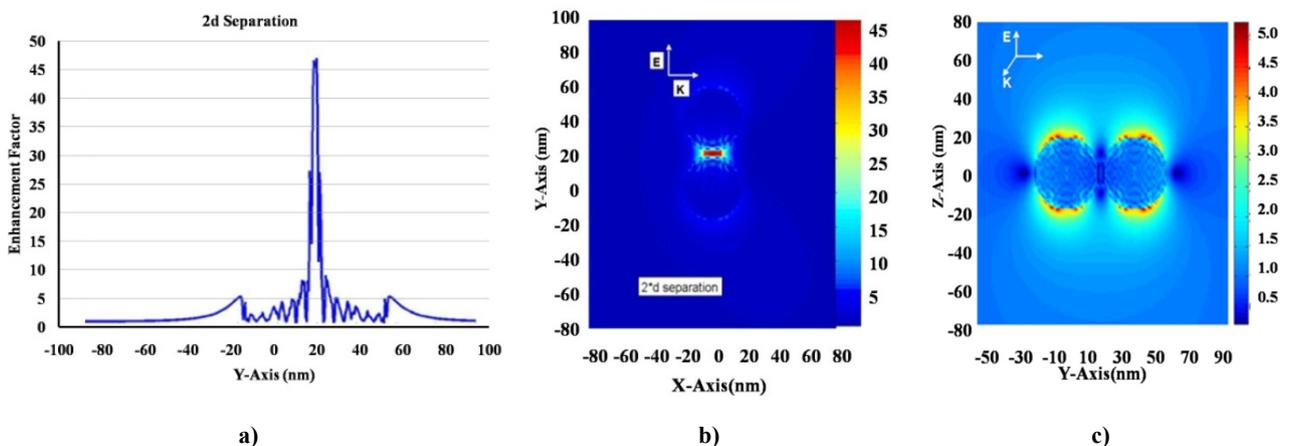
**Figure 5.** Electric field patterns (5b & 5c) and its magnitude (5a) along Y-axis of a doublet of 20 nm radius sphere separated about 2 nm (2\*d, d = 1.1 nm)
