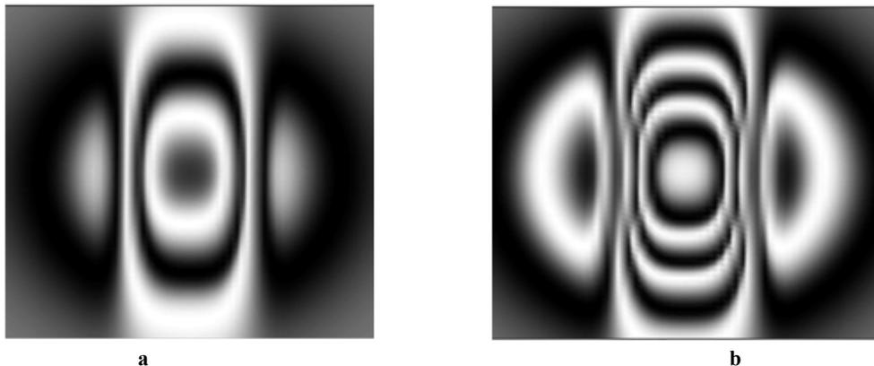
**Figure 3.** Changes in interference patterns at different exposures on photorefractive ones in LiNbO<sub>3</sub>:Fe crystals
