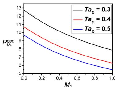
**Figure 8.** Variation of  $R_{D_c}^{osc}$  with  $M_1$  for  $F_1 = 1.5$ ,  $Va = 2$ ,  $F_2 = 0.3$ ,  $G = 0.06$  and  $M_3 = 2$
