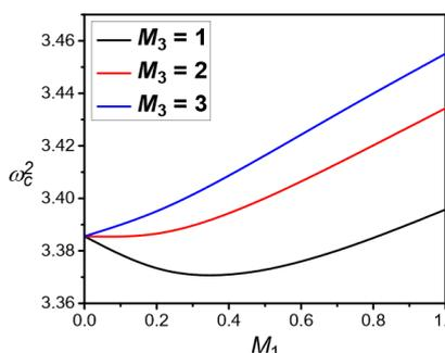
**Figure 12.** Variation of  $\omega_c^2$  with  $M_1$  for  $F_1 = 1.5, Va = 2, F_2 = 0.3, G = 0.06$  and  $Ta_D = 0.4$
