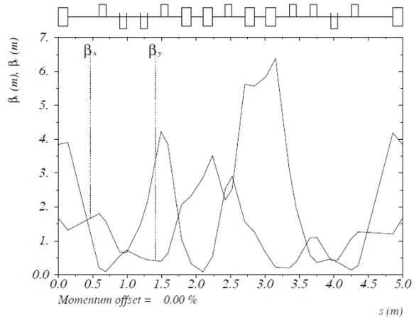
Fig. 5. Focusing functions  $\beta_x$ ,  $\beta_y$  by the channel beam injection
