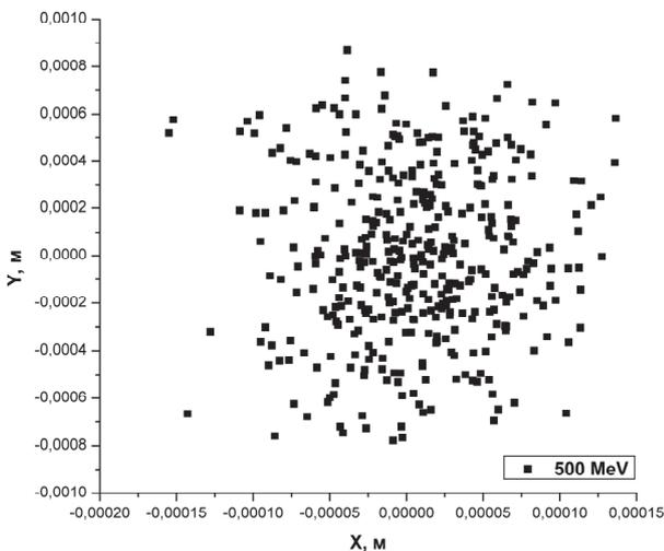
Fig. 23. Beam sizes on the second ring of recirculation (on magnet 12M10 exit) with sextupole component equal 0
