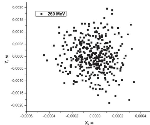
Fig. 10. Beam sizes on an entry in the first arch
