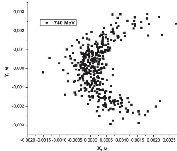
Fig. 24. Beam sizes at the maximum energy on an entry in 12M1 magnet
