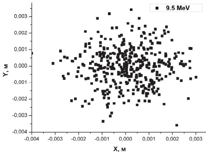
Fig. 2. Traversal cross-section of an injected beam
