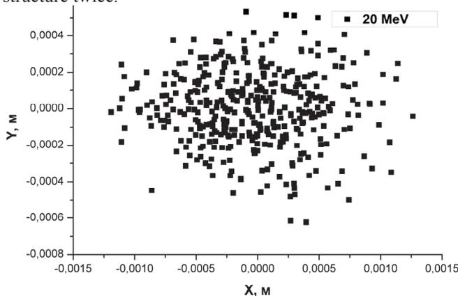
Fig. 9. Beam sizes on an entry in the basic accelerating structure
