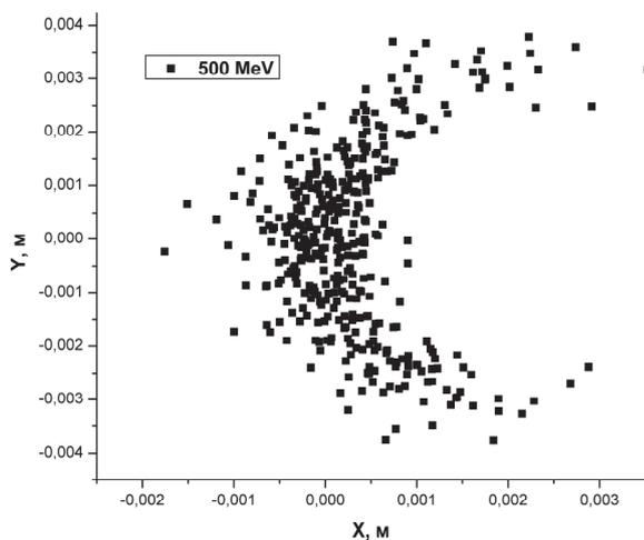
Fig. 19. Beam sizes on the second ring of recirculation (on magnet 12M5 exit)
