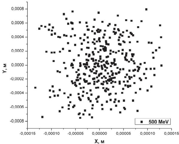
Fig. 21. Beam sizes on the second ring of recirculation (on magnet 12M10 exit)
