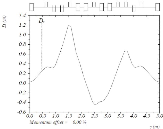
Fig. 6. Dispersion function  $D_x$  of the channel of injection
