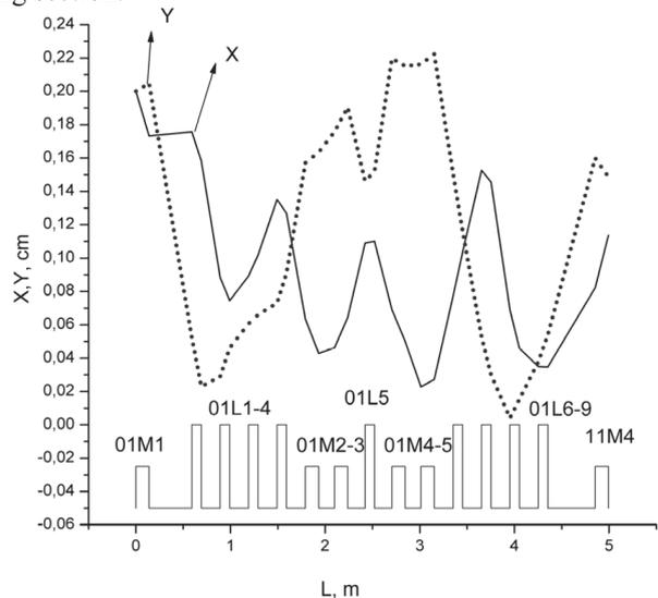
Fig. 7. Beam envelopes on a transportation section
