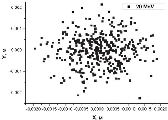
Fig. 4. The cross-section of the injection beam
