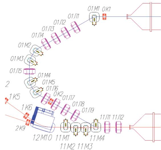
Fig. 3. Structure of the channel beam injection
