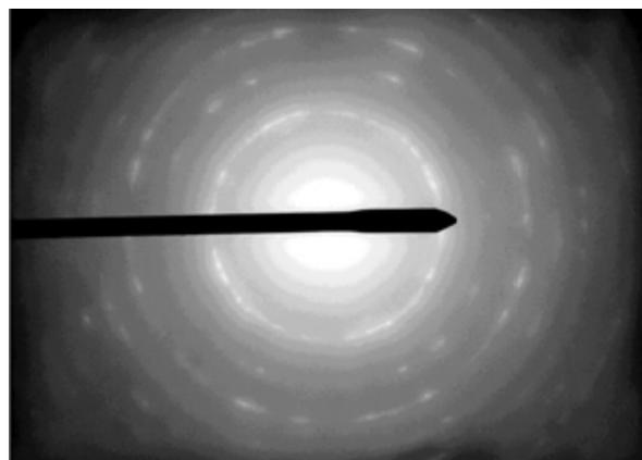
Fig. 9. Microdiffraction pattern of W coating (stl.st + Cu + W (μm)) composition.
