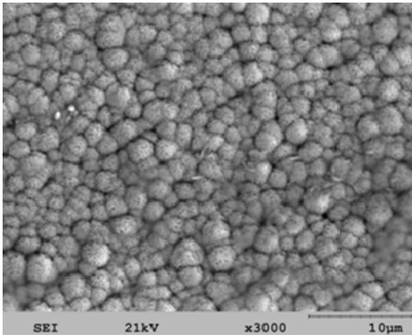
Fig. 4. Copper film on the overheating object.
