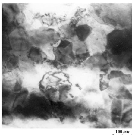
Fig. 8. Electron microscope image of W coating (stl.st + Cu + W (μm)).
