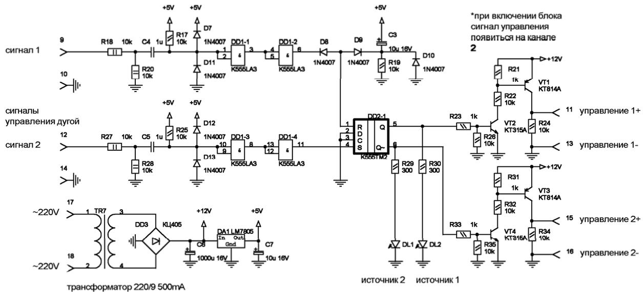
Fig. 3. Diagram of commutation of arc power supply unit
