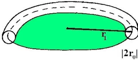
Fig. 2. Dislocation loop with the phason trail inside.
