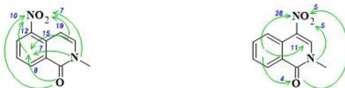
Figure 3. Excited state electron density redistribution at long-wavelength electronic transitions of nitro-isocarbostyrils (ESSA approach, charge-transfer numbers [% of electron charge]).
