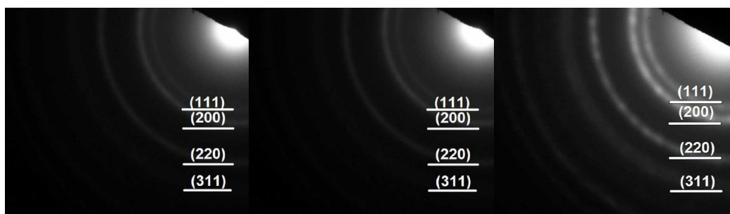
Figure 2. SAED images of the NiO films annealed at a – 250 °C, b – 300 °C, c – 600°C
