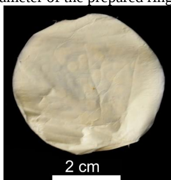
Fig. 2. Photo of samples of polymer nanofiber mat with incorporated AgNPs.
