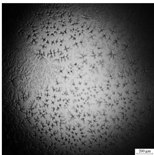
Figure 11. The film from the solution containing 0.4 mM ZnCl 2 and 10 mM NaCl. T=40°C, H=18%.
